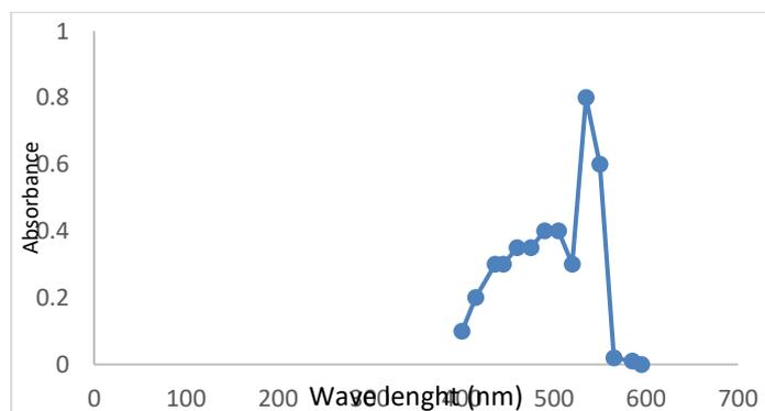
Figure 1. The UV/VIS Spectrophotometric scan of pigment produce
